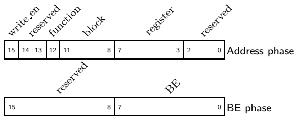
Figure 1: Address and BE phases for register access
