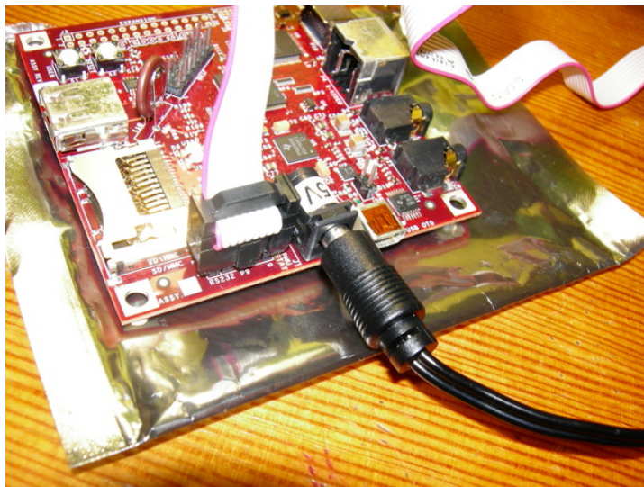
Figura 3.11: Board power supply connection
