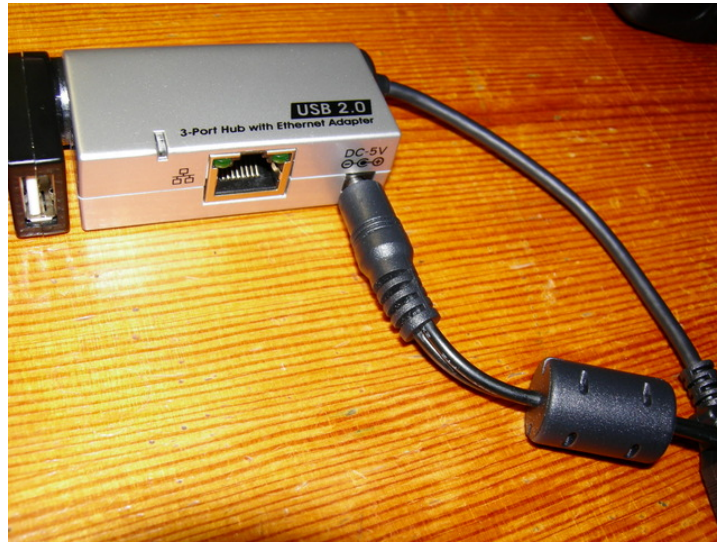
Figura 3.8: Hub connected to power supply
